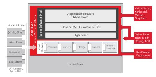
Figure 1. Simulate your entire target system
