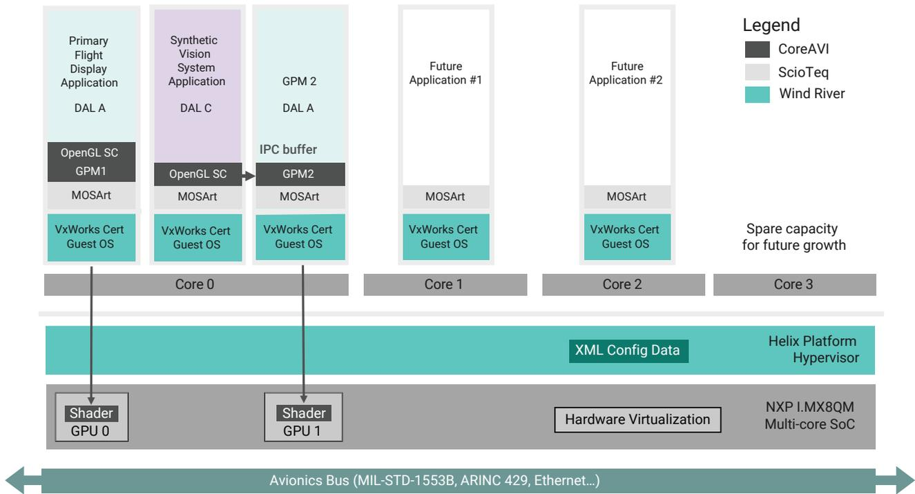
Figure 12. ScioTeq display platform architecture with example configuration
