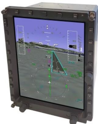
Figure 13. MFD-5068 multi-function display (Source: ScioTeq)
