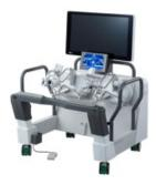
Figure 1. Saroa uses a standard flat-panel display rather than an immersive monitor, facilitating communication for the human surgical team
