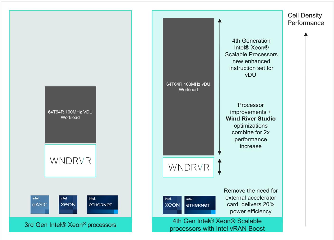
**Figure 5.** Performance results from the Wind River Studio tests (higher is better) The 3<sup>rd</sup> Gen Intel® Xeon® Scalable processors support 20 radios on two cores, whereas the 4<sup>th</sup> Gen Intel® Xeon® Scalable processor supports 32 radios on one core.
