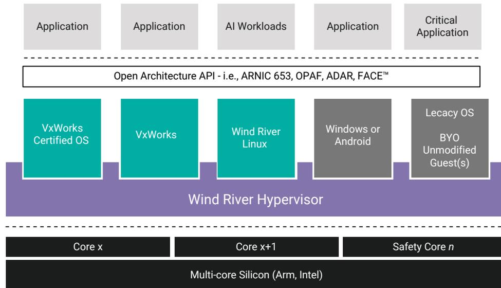
Figure 2. Example of an open architecture hypervisor running multiple OSes
