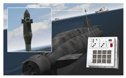
from the submarine fin and rapidly perform a 360-degree scan of the surface above, enabling the commander to analyze the image data afterward, minimizing the risk of detection. The SHU is a pressureproof, electro-optical assembly that contains high-performance cameras, optics, environmental sensors, and stabilization mechanisms. It is designed to function in temperatures ranging from minus 15 C to more than 60 C and withstand nearby explosion.
