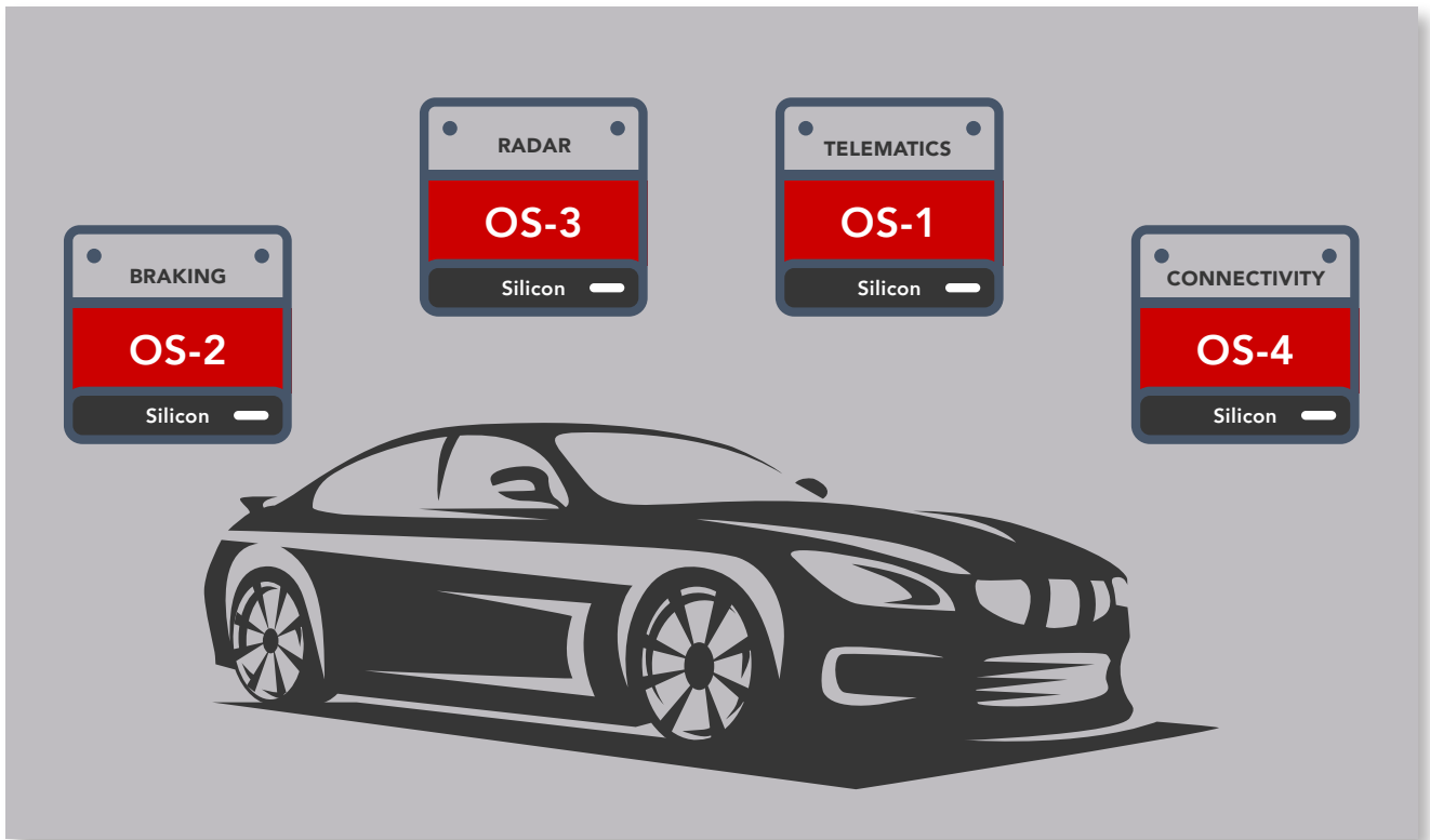
Figure 1 – Examples of multiple, separate, and proprietary embedded systems running on a car
